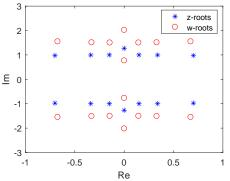
The patterns of z-roots (blue asterisks) and w-roots (red circles) in complex plane at the ground state with N = 6,  $\eta = i$ , p = -1.2i,  $\bar{q} = 0.8i$ ,  $\xi = 1$ ,  $\{\theta_j = 0\}$ .
